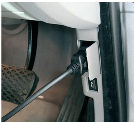
Autologic attaches simply via the diagnostic port – the ECU doesn't need to be physically removed. Graphs show big gains – power on the left and torque on the right
